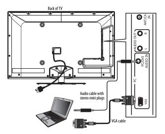
3 Connect an audio cable with stereo mini plugs to the PC/DVI AUDIO IN jack on the side of your TV and to the LINE OUT or AUDIO OUT jack on the computer.
